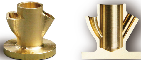
Drilling a parabolic shape by machining with 5-axis simultaneous control
