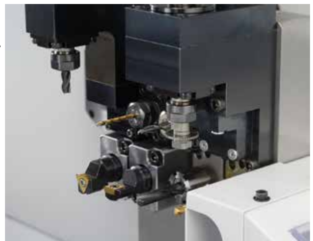
The back tool post on Type X and XII machines can accommodate a total of 8 tools: 4 rotary tools in the upper row and 4 fixed tools in the lower row.
