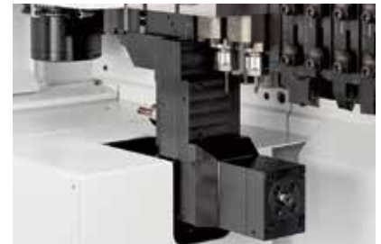
During B-axis tool change
