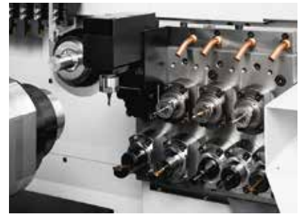
U12B (Back tool post incorporating Y axis)
