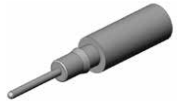
Connector pin (1.5 mm dia., L = 10 mm)
