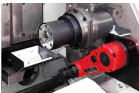
Part catcher Catches workpieces without damaging them and transfers them to the part conveyor.
