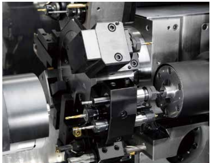
Back machining using tools installed in a triple sleeve holder
