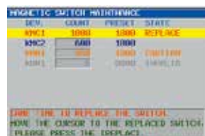
Electromagnetic switch maintenance
