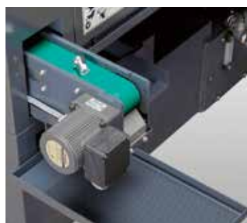
Part conveyor Transports workpieces received from the part catcher to outside the machine.
