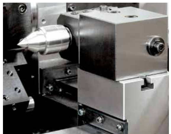
Tailstock (live center, MT2)
