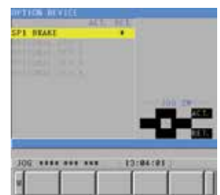
Option device Used to select an auxiliary device such as a part catcher to be operated manually.
