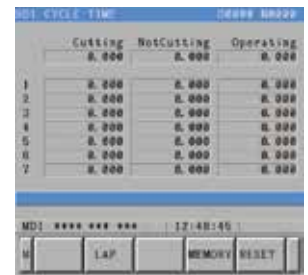
Cycle time Measures the cutting time, non-cutting time and running time in each cycle.
