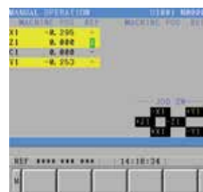
Manual operation Displays the zero point lamp status and the machine coordinate of each axis.
