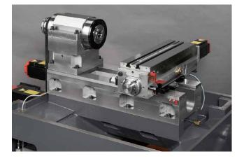
The supply of lubricating oil to a slideway results in a very slight lift and yawing, affecting machining accuracy to a very small degree. The use of "program-controlled lubrication", which enables control matched to cycle times, makes it possible to generate an oil film of the ideal thickness and achieve stable high accuracy.
