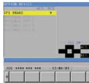
OPTION DEVICE Used to select an auxiliary device such as a part catcher to be operated manually.
