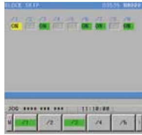
BLOCK SKIP Used to set block skip 1 to block skip 9.
