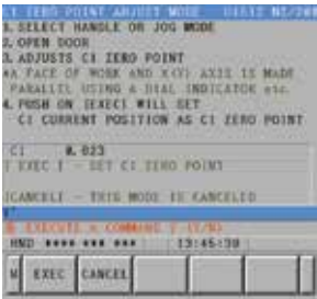
C Zero point adjust mode Easy to adjust the C axis zero point.
