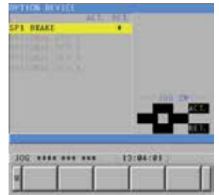
Option device Used to select an auxiliary device such as a spindle brake to be operated manually.
